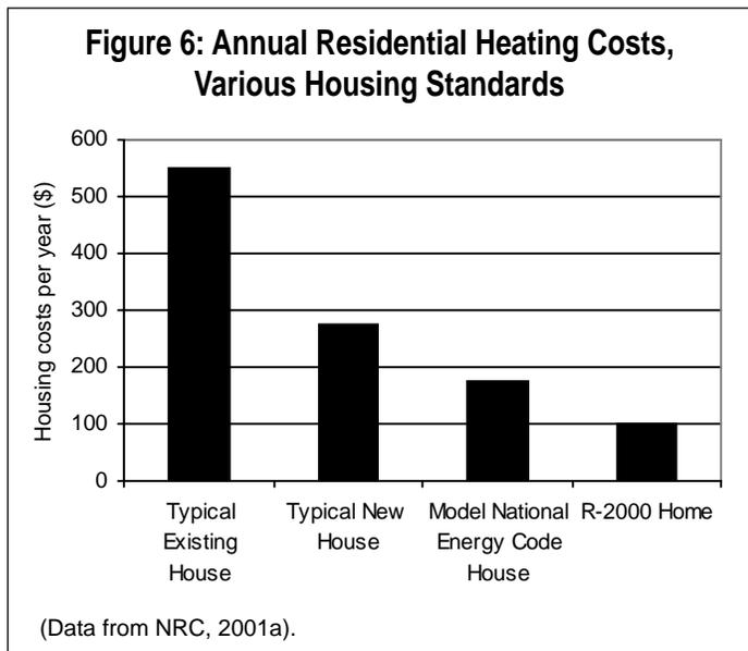
Energy use in the residential and commercial sectors is greatly affected by the building standards applied to their construction. For example, Figure 6 illustrates the huge variation in heating costs for homes built under different building standards. This speaks both, to the need to improve upon existing building codes, and to encourage retrofits for existing buildings.
